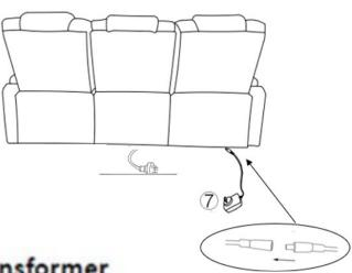
Safety Note: Transformer and cables are not to be placed under or within the recliner structure.
